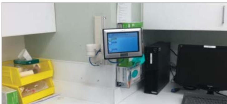
*A DOCS® touchscreen interface for the M2 is shown, remotely mounted at the circulator's desk, and near their HIS terminal. This option is available for those that do not desire to have the DOCS touchscreen monitor mounted in the standard configuration on the side of the NuBOOM cabinet.*
